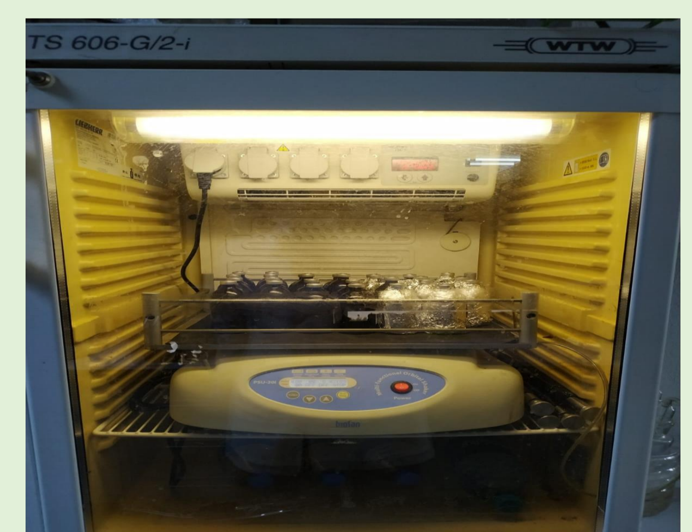
Figure 4. Incubator used to keep the temperature of BMP test bottles at 35°C
